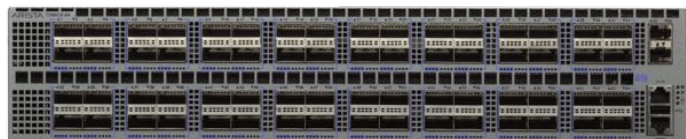
Arista 7260CX-64: 64 x 40/100GbE QSFP100ports, 2 SFP+ ports
